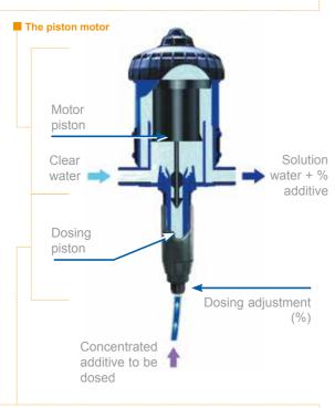
Therefore, the operating principle ensures constant dosing, independently of the variations in flow rate and pressure of the
